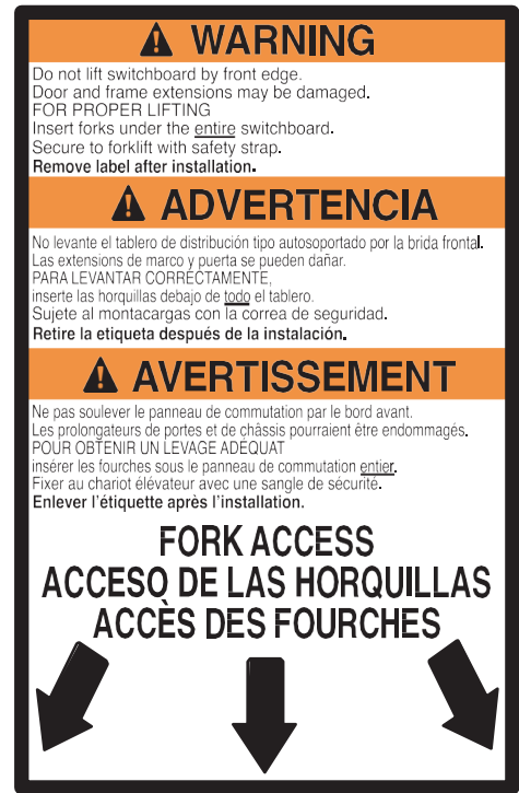
Figure 4: Warning Instruction Label, Rainproof Switchboards
